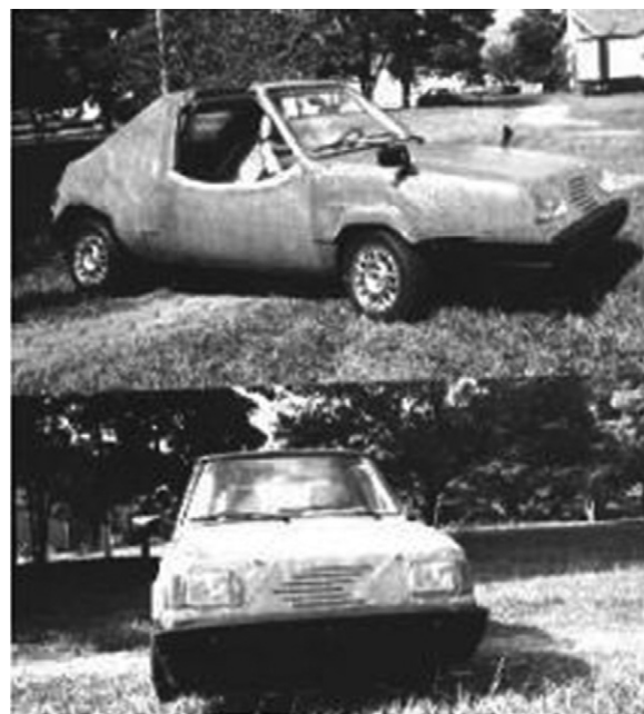
Fig. 2. A car made from jute fibre reinforced composite and hybrid composite in Brazil (with permission).
